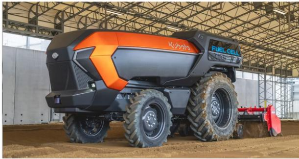
Kubota's new concept tractor has dual motors, one for drive and one for implements, and can self-drive to the field. Source: Kubota Corp.
