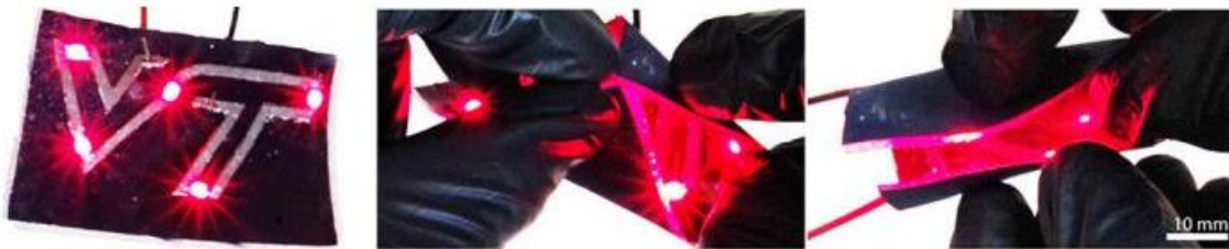
This ironed-on circuit creates a “VT” pattern that lights up LEDs, even when bent into different shapes (as shown in the middle and right images).
