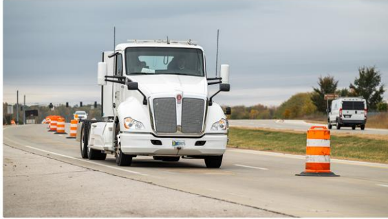
An electric Cummins heavy-duty truck charges as it drives along a test segment on U.S. Highway 52/U.S. Highway 231 in West Lafayette. (Purdue University photo/Kelsey Lefever)
