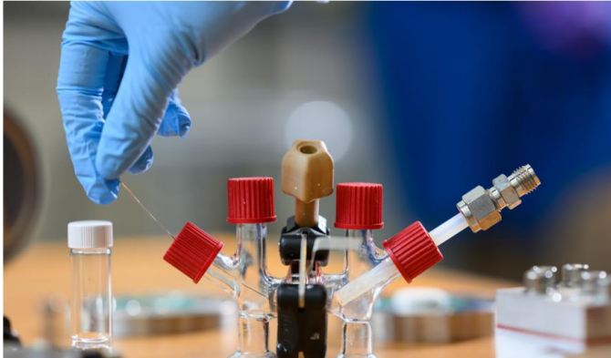
An H-cell modified with electrodes and an ion-conducting ceramic membrane to conduct sodium-air fuel cell experiments.
