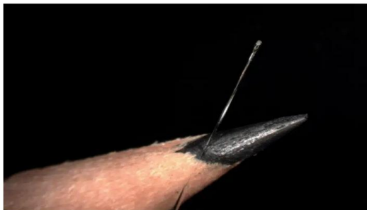
Researchers use a very thin optical fibre for 3D printing. The image shows the fibre in comparison to a pencil lead.
