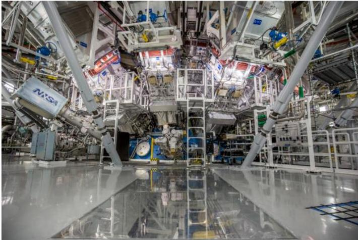
The target chamber of LLNL's National Ignition Facility, where 192 laser beams delivered more than 2 million joules of ultraviolet energy to a tiny fuel capsule to create fusion ignition on Dec. 5, 2022. (NIF Photo)
