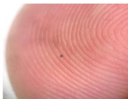
A microbot, fully integrated with sensors and a computer, small enough to balance on the ridge of a fingerprint.
