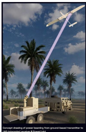
Concept drawing of power beaming from ground-based transmitter to UAS-integrated receiver © PowerLight
