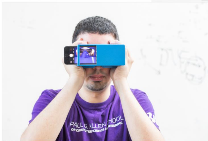
BiliScreen is a new smartphone app that is designed to screen for pancreatic cancer by having users snap a selfie. It's shown here with a 3-D printed box that helps control lighting conditions to detect signs of jaundice in a person's eye. Dennis Wise/University of Washington
