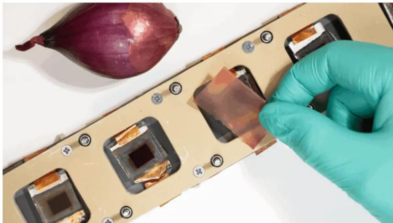
📷 A film dyed with red onion skin extract and dye-sensitised solar cells. The films were placed on top of the solar cells in the study. Credit: Väinö Anttalainen
