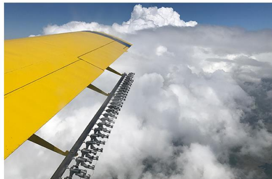
An airborne plane sports the nozzles used to spray the charged particles. (Photo courtesy of Daniel Martin, D4963-1)
