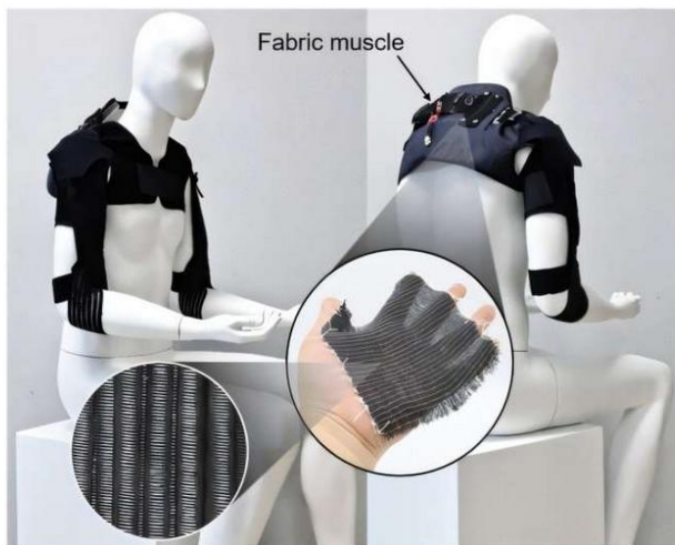
Conceptual design of the proposed soft and simple shoulder joint assistive exosuit, featuri
