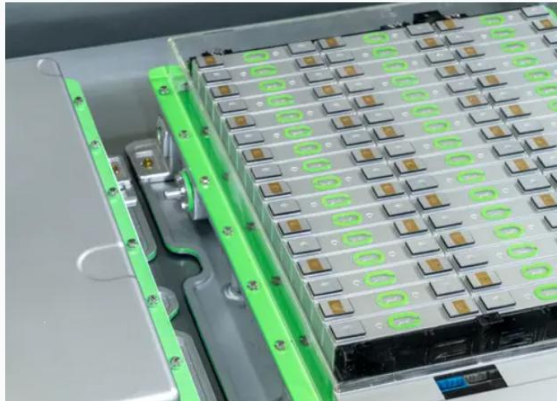
The ETOP system streamlines this process by stacking sealed anode and cathode pairs directly into the battery pack. (Representational image) zhihao/Getty/images
